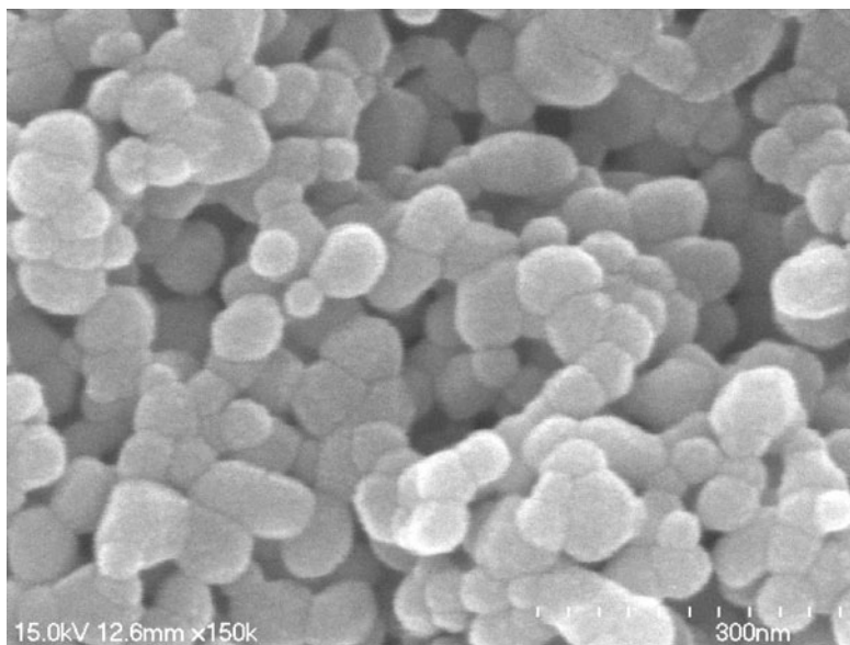
Figure 3. FE-SEM images of \text{ZnGa}_2\text{O}_4 phosphor prepared at 1000^\circ\text{C} .
